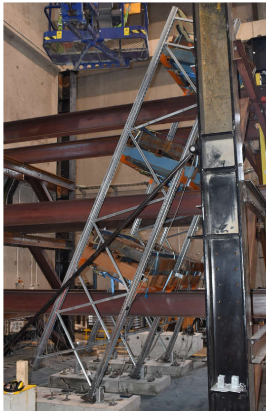
Figure 10: Unanchored baseplate frame overturned at design level 1.5x Northridge earthquake
