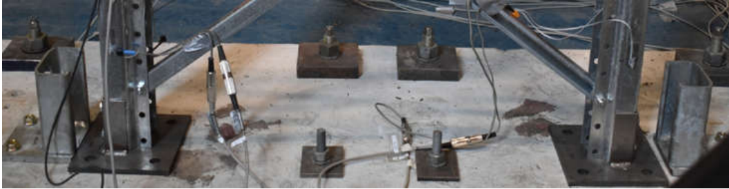
Figure 9: Unanchored baseplate: Restraining cross-aisle movement while allowing frame uplift
