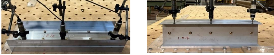
Figure 3: Test setups for initial local geometric imperfection measurements.
