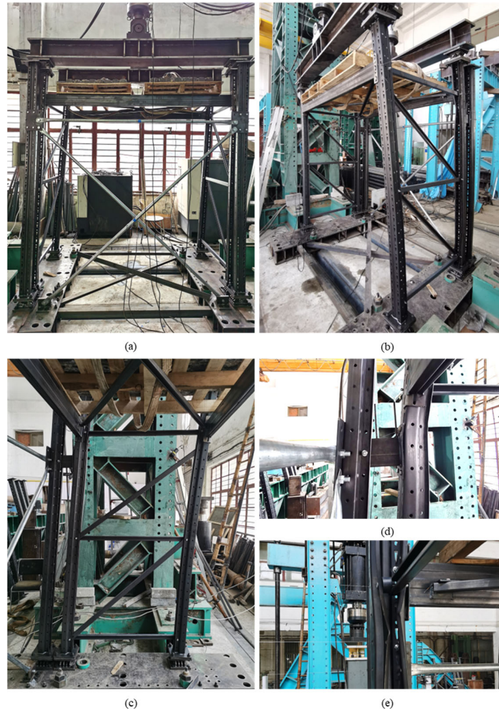
Figure 7: Sway and failure mode of a representative tested rack frame.
