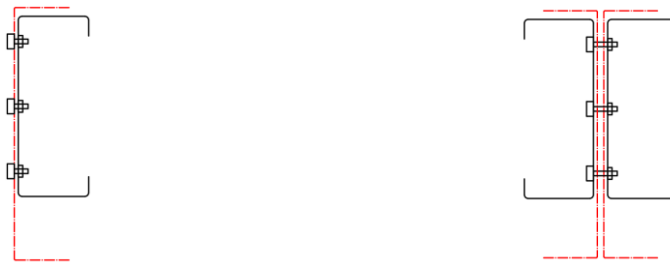
(a) One bracket and one channel (1B1C) (b) Two brackets and two channels (2B2C)
