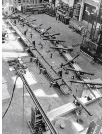
Figure 5: Full-scale portal frame test after Lim and Nethercot [1].
