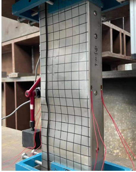
Figure 4: Failure mode of stub column specimen HA-CC-S4.
