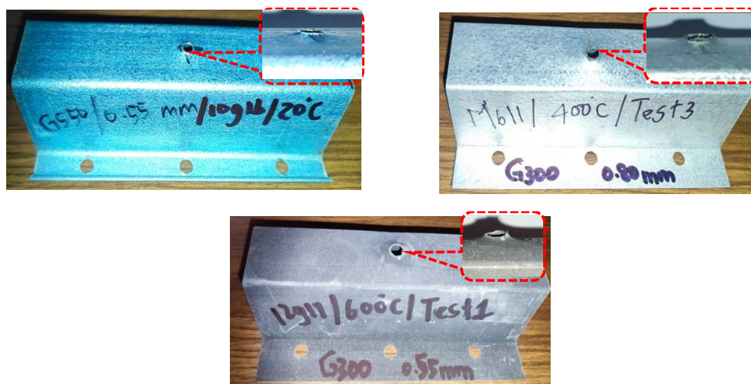
Figure 5: Permanent deformations on battens during pull-out
